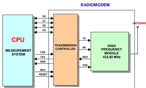
Fig. 3. Radiomodem block diagram
