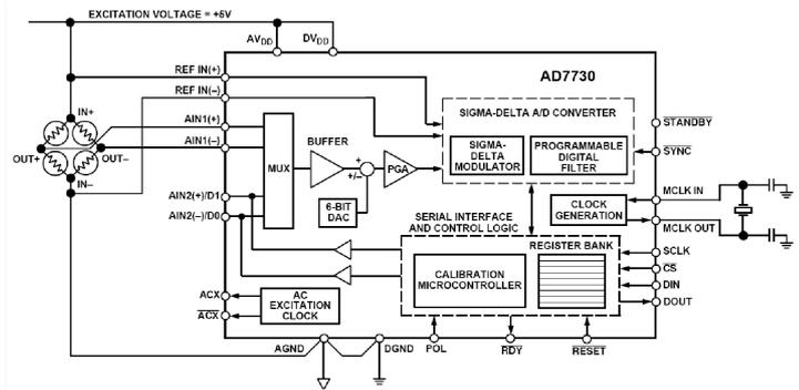
Fig. 2. Simplified block diagram of the strain gauge measurement circuit [1]
