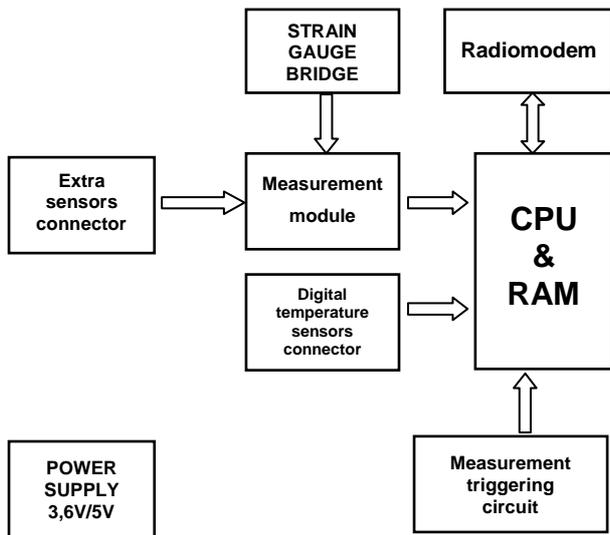
Fig. 1. Conditioner block diagram
