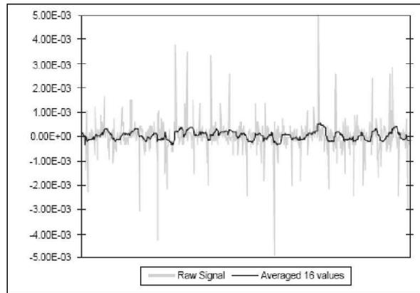
**Fig. 6.** Noise reduction using averaging [5]
